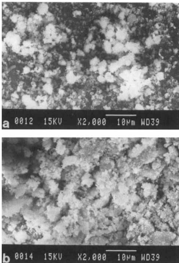
FIG. 9 SEM microphotographs of the studied hydroxyapatite: (a) HAP without any treatment or contact with water; (b) HAP dispersion (1 g/L concentration) in aqueous solution without cadmium, and (c) in the presence of 10 mg/L Cd (contact time 900 seconds). Both samples (b) and (c) were filtered through a 0.45- \mu\text{m} membrane and dried at room temperature.
